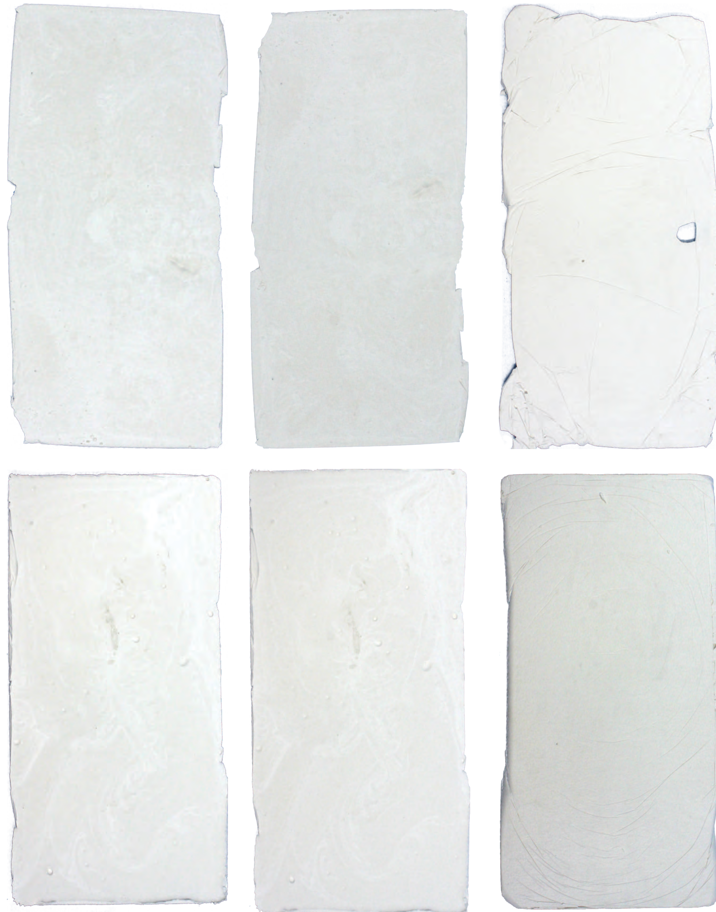
Plaster panels of varying thicknesses were produced to test the limits of the material in this form. Some panels broke whilst being removed from their moulds. Others could survive being dropped to the floor
